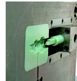
Core mold insert assembled to the mold base.
